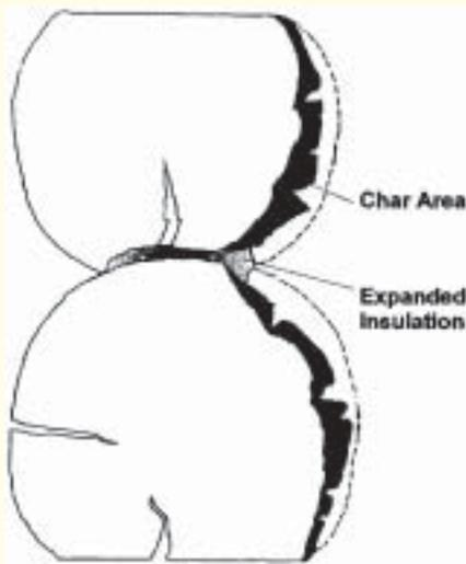
*Cross section of log wall after fire test. The mineral wool insulation in the long groove expanded, once the edge of the groove burned off. The insulation created a protective shield against heat penetration through the wall joint.*
